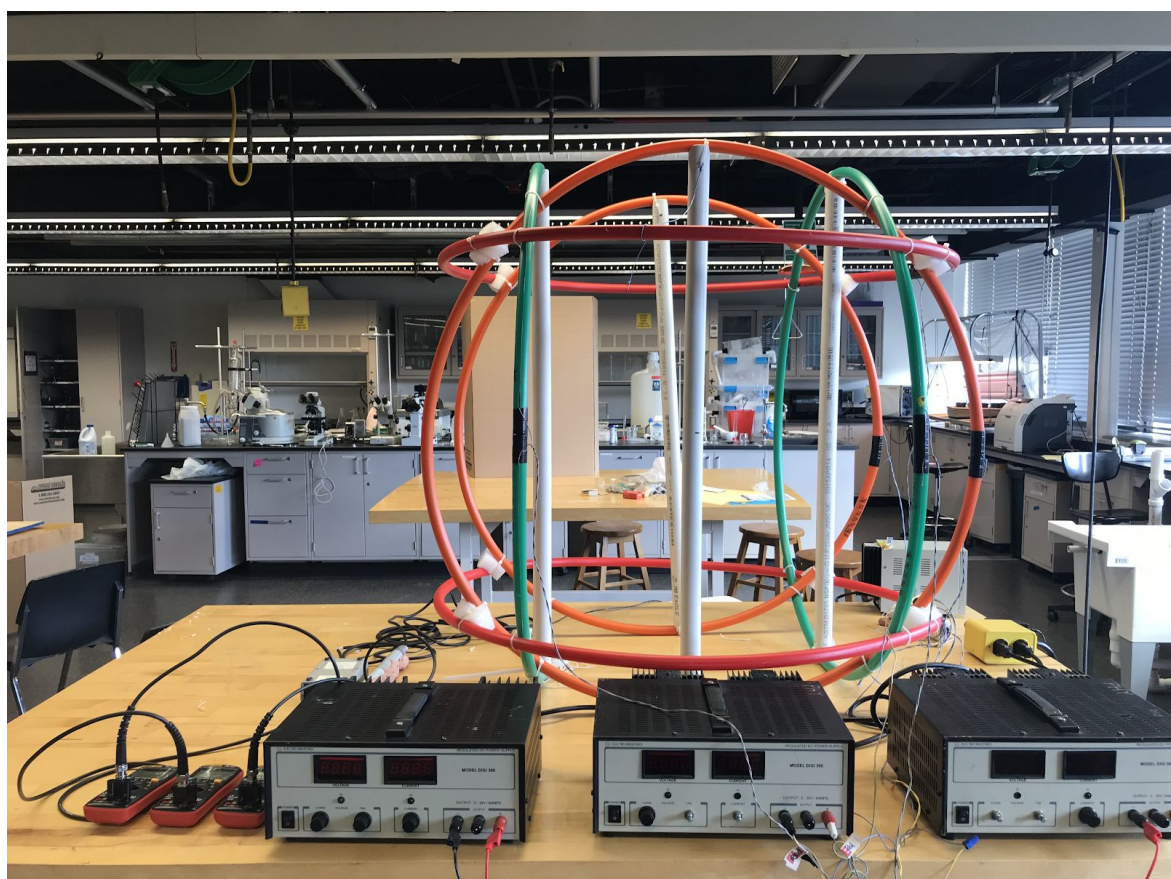
Figure 3. Hoopla system used to cancel out Earth's geomagnetic field in the training environment
